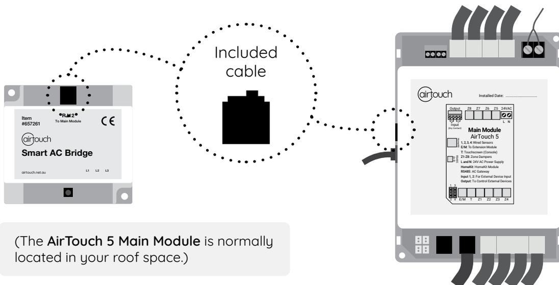
Note: The **AirTouch 5 Main Module** will provide power to the **Smart AC Bridge** over the cable when connected.
